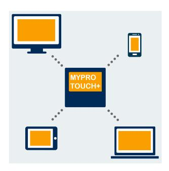
The MYPRO TOUCH+ also offers options to remotely monitor the HMI from a smart phone or tablet. Combine this feature with a VPN access to your network and you can have 24/7/365 access to your MYPRO TOUCH+. Simply download a VNC viewer app to your smart device and connect to the IP address of your MYPRO TOUCH+ panel in your network.
